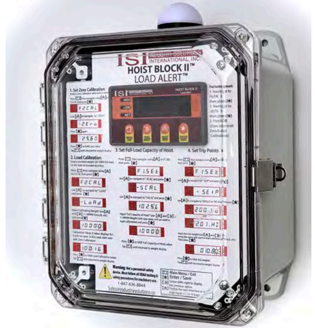
fig1. Hoist Block II™ (HB2) is a hoist load limit controller used with either an ISI Rope Load Cell or the ISI Load pin. 11.04 x 9.04 x 9.72 inches, 115VAC/230VAC powered (other available including 230 vdc or vac etc. NEMA 4X IP68 Polycarbonate with 2 form C relays for HIGH and LOW trips (Low can be used for Slack Rope). Can be placed on the hoist itself or where easily viewed. The dome on the top is a red/green visual indicator with audible alarm.
